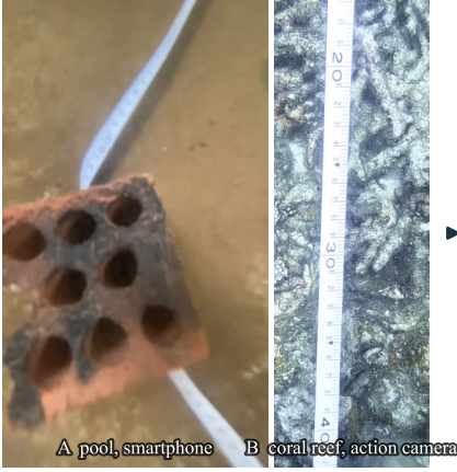
Fig. 1. Workflow and problems of metric monocular transect mapping. (a) A single camera records the transect tape in a pool and on a coral reef. (b) Four problems prevent a direct use of the tape as a metric reference. P1 is the unknown and drifting scale of a monocular reconstruction. P2 is the bend of the tape over the relief, which makes the chord shorter than the material length. P3 is the weak image evidence of the tape interior. P4 is the break of a long sequence into several models. (c) RIFT-Map resolves them in one metric map whose tape intervals keep their material lengths.
